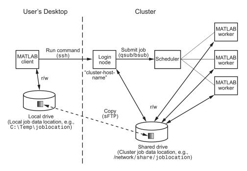
In this type of configuration, job data is copied from the client host running a Windows operating system to a host on the cluster (cluster login node) running a UNIX operating system. From the cluster login node, the LSF bsub command submits the job to the scheduler. When the job finishes, its output is copied back to the client host.
